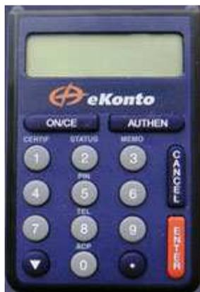
1. Switch on Personal Electronic Key (ON/CE), insert PIN and press ENTER button twice.
