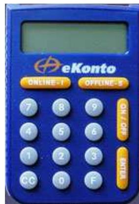
1. Switch on Personal Electronic Key (ON/OFF), insert PIN and press ENTER button.
